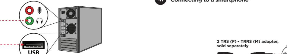
**ATTENTION:** background noise appears if the electrical circuit is poorly shielded on the computer. In this case, connect the USB plug to the USB adapter (not included in the package).
